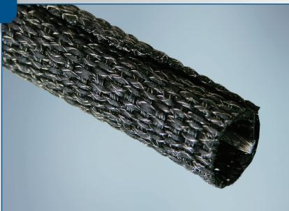
**TwistTube® 2472** is a self-wrapping sleeve designed to provide >30dB of electromagnetic (EM) screening attenuation. 316L fine stainless steel wire is combined with polyester yarn to create a wrappable product that offers flexibility and consistent shielding protection in corrosive environments. The product features an acrylic/silicone coating to prevent end fray and enable cold cutting for specific product lengths.
