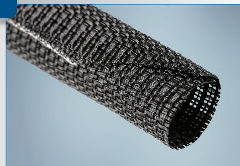
**TwistTube® 2439** is a high temperature, lightweight woven sleeve designed to provide mechanical protection for cable assemblies, hoses and wire harnesses. It incorporates a unique self-wrapping closure that allows for quick and easy installation. It also allows for breakouts and can be installed over complete assemblies. The overwrapping design of the product allows it to maintain a circular profile when flexed.
