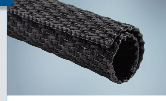
**TwistTube® 2426** is a self-wrapping sleeve designed to provide excellent edge abrasion protection and noise suppression. Woven of both monofilament and multifilament polyester yarns the product offers a high level of component protection and is both flexible and lightweight. The polyester construction eliminates problems associated with trapped heat and humidity and also eliminates operator skin irritation during assembly.
