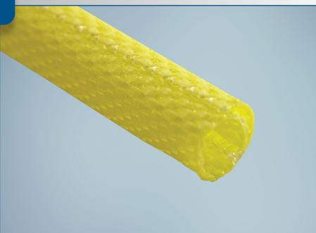
**TwistTube® 2425F** is a self-wrapping sleeve designed to provide mechanical protection and acoustical noise suppression. Woven of both monofilament and multifilament polyester yarns the product offers a high level of component protection and is both flexible and lightweight. Colored yellow, TwistTube 2425F is commonly used to identify critical assemblies such as airbags.
