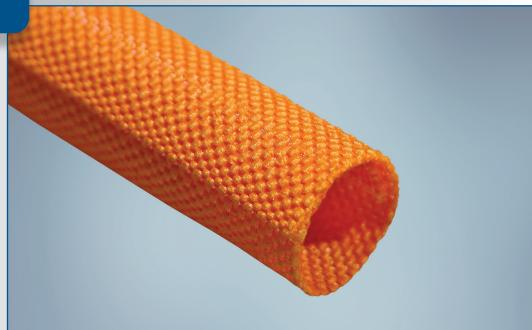
**TwistTube® 2424** is a self-wrapping sleeve designed to provide mechanical protection and acoustical noise suppression. Woven of both monofilament and multifilament polyester yarns the product offers a high level of component protection and is both flexible and lightweight. Colored orange, TwistTube 2424 is commonly used to identify high voltage cables in hybrid vehicles.
