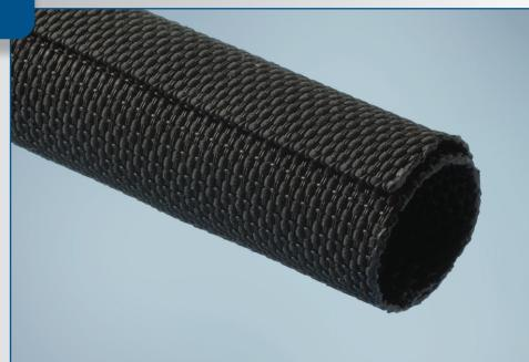
**TwistTube® 2421** is a self-closing oversleeve designed to provide mechanical protection and to suppress acoustic noise. Woven of monofilament and multifilament polyester yarns the product offers superior abrasion protection, high level of component protection and is both flexible and lightweight. Its unique construction eliminates problems associated with trapped heat and humidity.
