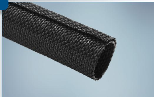
**TwistTube® 2420F** is a self-wrapping sleeve designed to provide abrasion protection and acoustical noise suppression. Woven of both monofilament and multifilament polyester yarns the product offers a high level of component protection and is both flexible and lightweight. The polyester construction eliminates problems associated with trapped heat and humidity and also eliminates operator skin irritation during assembly.
