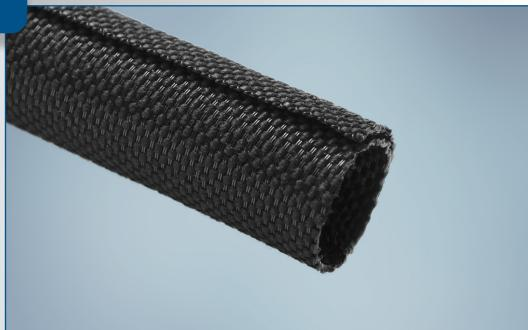
**TwistTube® 2420** is a self-wrapping sleeve designed to provide abrasion protection and acoustical noise suppression. Woven of both monofilament and multifilament polyester yarns the product offers a high level of component protection and is both flexible and lightweight. The polyester construction eliminates problems associated with trapped heat and humidity and also eliminates operator skin irritation during assembly.
