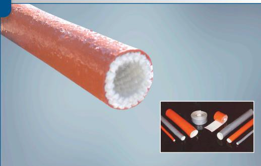
**Thermotubix**<sup>®</sup> is a thickwall braided fiberglass sleeving coated with a specially compounded, flame retardant silicone rubber. This product can be easily installed on cables and hoses and expands to pass over fittings and couplings.
