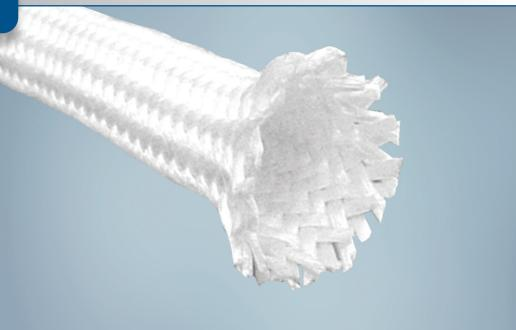
**Thermojacket® T** is constructed of braided high bulk fiberglass yarn. These yarns provide a heavier wall thickness with only a modest weight increase over other Thermojacket products. Thermojacket T provides excellent insulation properties and withstands continuous heat exposures to +538°C (+1000°F).
