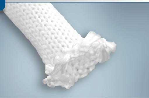
**Thermojacket P** sleeving is an unsaturated bulky knit constructed of high-temperature fiberglass yarn that withstands temperatures up to +760°C (+1400°F) in continuous operation. Use of this product offers an especially cost-effective application for resistance to high temperatures.
