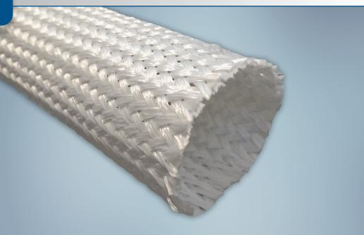
**ThermoJacket® C** is an uncoated, unsaturated sleeving braided from Nextel\* 312 ceramic fibers. ThermoJacket C retains strength and flexibility at continuous temperatures up to 1204°C (+2200°F) and offers significant protection against short term exposures at +1426°C (+2600°F).
