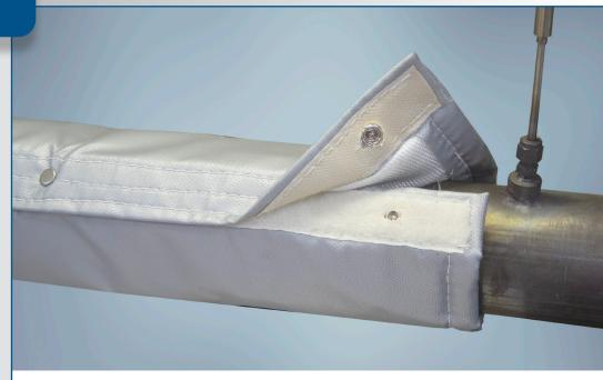
ThermShield™ 1231 is a multi layer thickwall wrappable sleeving developed for insulation of high temperature exhaust systems. Mainly used in engine compartment for high temperature control such as EGR, manifold and turbo, also in exhaust system to improve gas emission such as SCR, PDF and EGP.
