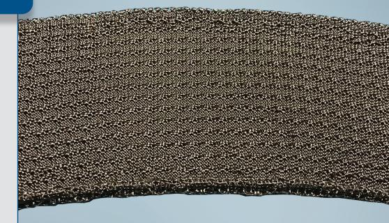
**ThermShield™ 1229** is a knitted fabric developed for insulation of high temperature exhaust systems. Designed with basalt yarns, ThermShield 1229 can withstand temperatures up to +750°C (+1382°F).
