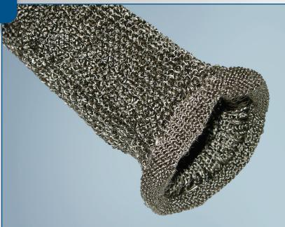
**ThermFlex® 1224** is a knitted sleeve developed for insulation of high temperature exhaust systems. Designed with basalt yarns, ThermFlex 1224 can withstand temperatures up to +750°C (+1382°F).
