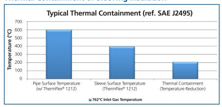
Note: Thermal Containment = Pipe Surface Temperature - Sleeve Surface Temperature.
