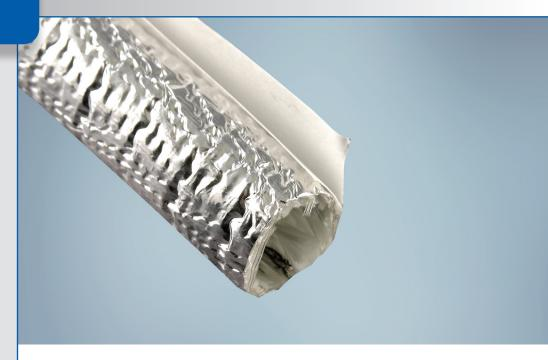
**Therm-L-Wrap™66** is a self-wrapping, reflective sleeve designed to provide thermal protection from both radiant and convective heat. Composed of a woven fiberglass base fabric and a lamination of aluminum foil, the product can withstand convective heat soaks up to 200°C and simultaneously protect critical components from radiant or reflected heat.
