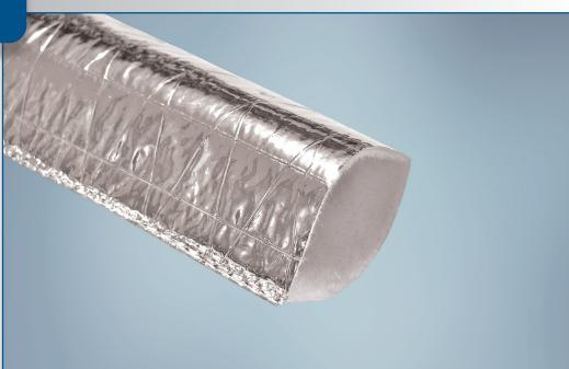
**Therm-L-Lite**<sup>®</sup> is reinforced, aluminized polyester sleeve designed to protect components in high temperature environments. The external surface is composed of a highly reflective aluminum foil, which provides radiant heat protection for internal components. The internal layer is composed of a polyester non-woven material, which provides added insulation efficiency. A layer of fiberglass scrim contributes to both product flexibility and durability.
