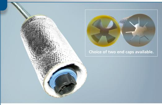
**Therm-L-Gard<sup>™</sup> V** is an aluminized, high bulk sleeve designed to provide thermal protection in high temperature environments. The outer layer is composed of an aluminum and glass fabric with the inner layer being composed of non-woven polyester.
