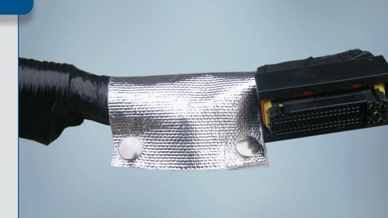
**Therm-L-Gard™ S** is a flexible, aluminized, wrappable sleeve designed to protect components in high temperature areas. The outer aluminum finish is highly reflective while the inner layer of fiberglass greatly increases insulating efficiency.
