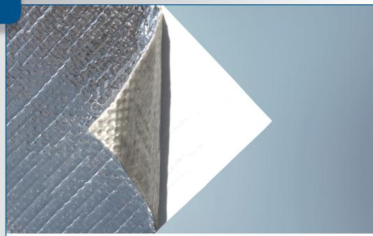
**Therm-L-Gard™ A** is a woven fiberglass fabric with aluminum foil laminated to its outer layer and a pressure sensitive adhesive on the inner layer. The unique multipolymer adhesive exhibits high adhesion to low surface energy plastics such as HDPE, polypropylene and gas filled polypropylene.
