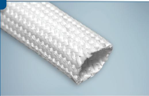
**TST/TSX** is a high temperature resistant, multifilament pure silica fibre (>99,8%) braided sleeving. It has a continuous working temperature of  $-60^{\circ}$ C to  $+950^{\circ}$ C.
