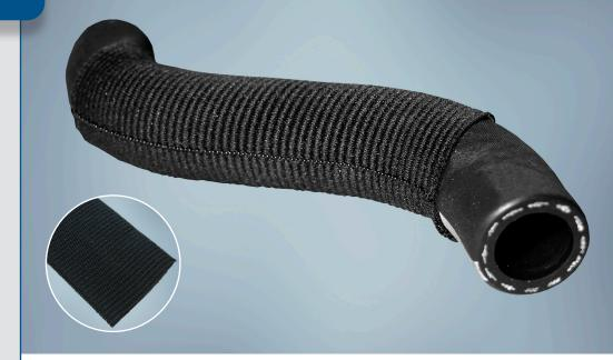
ShrinkGard™ 2800 is a highly flexible, woven sleeve constructed of polyester and polyethylene that provides good abrasion resistance for rubber hoses and tubing applications. The product offers a shrinkage up to 60% which allows ShrinkGard 2800 to accommodate a variety of diameters and sizes. The soft construction of ShrinkGard 2800 is ideal when handling the product during installation.
