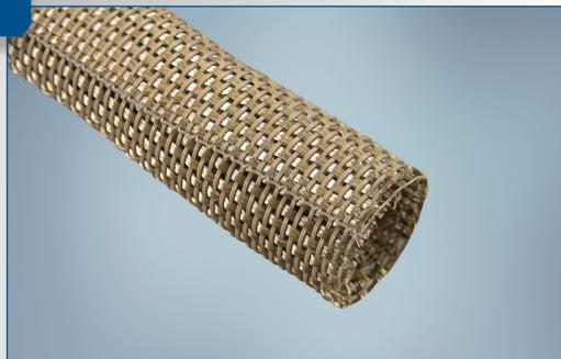
**ROUNDIT® V0 EMI Cu/Sn** is a wrap-around sleeving designed for high performance EMI shielding of wire and cable bundles. ROUNDIT V0 EMI Cu/Sn is manufactured from UL 94 V0 rated PPS monofilaments and tin plated copper wires according to EN13602.
