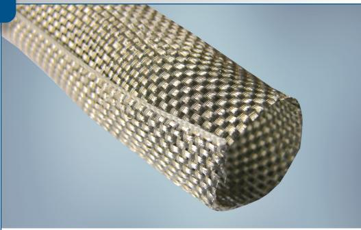
**ROUNDIT® V0 EMI** is a wrap-around sleeving designed for high performance EMI shielding of wire and cable bundles. ROUNDIT V0 EMI is manufactured from UL 94 V0 rated PPS monofilaments and nickel plated copper wires class 4 according to ASTM B-355.
