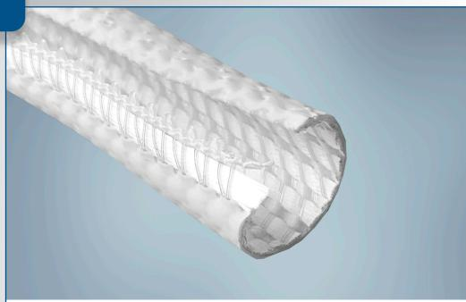
**ROUNDIT®** Therm-C is a woven sleeve coated with an intumescent coating designed to protect wire harnesses from the effects of thermal environments in excess of +230°C.
