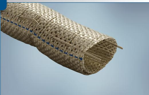
**ROUNDIT® EMI DW** is a wrap-around sleeving designed for high performance EMI shielding of wire and cable bundles. ROUNDIT EMI DW is manufactured from UL 94 VO rated PPS monofilaments and nickel plated copper wires according to ASTM B-355.
