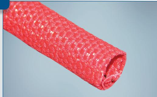
**ROUNDIT® 2000 NX Red** is a self-wrapping sleeve manufactured from PPS monofilaments and Nomex® with an oil and water repellent treatment, designed for mechanical protection and maintenance of wire and cable bundles. Its construction with 100% covering ratio provides excellent cut-through and abrasion resistance.
