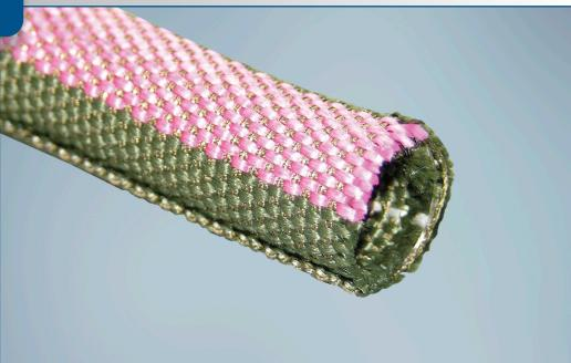
**ROUNDIT® 2000 NX Ptr** is a self-wrapping sleeve manufactured from PPS monofilaments and Nomex® multiflaments with a water repellent treatment, designed for mechanical protection and maintenance of wire and cable bundles. This design allows for 100% coverage providing excellent cut-through and abrasion resistance.
