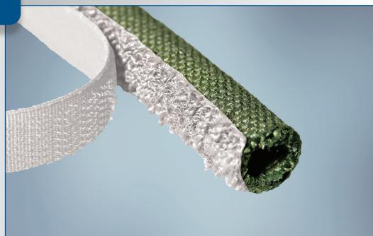
**ROUNDIT® 2000 NX GRIP** is a woven combination of Nomex® and PPS (polyphenylene sulfide). The Nomex/PPS blend in a flat weave construction gives ROUNDIT 2000 NX GRIP a rugged yet smooth texture and appearance for high temperature bundling and abrasion resistance. This product is rated to +200°C (+392°F) and is non-halogenated.
