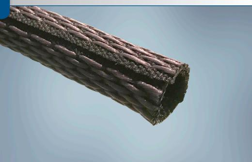
**ROUNDIT® 2000 FR GRIP** is a wrap-around sleeving manufactured from flame-retardant polyester monofilaments and multifilaments, designed for mechanical protection and maintenance of wire and cable bundles. Its construction with 100% covering ratio provides good abrasion resistance.
