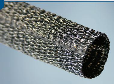
**ROUNDIT® 2000 Cu EMI** is a self-wrapping sleeve designed to provide >40dB of electromagnetic (EM) screening attenuation. Tinned copper wire is combined with polyester yarn to create a wrappable product that offers flexibility and consistent shielding protection. The product features an acrylic/silicone coating to prevent end fray and enable cold cutting for specific product lengths.
