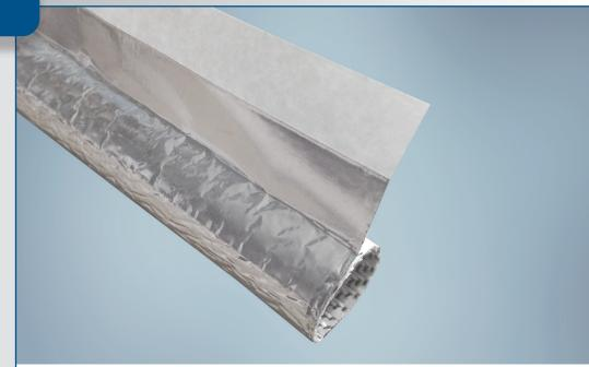
**ReflexWrap™ 1463 LF** is a self-wrapping, reflective sleeve designed to provide thermal protection for both radiant and convective heat applications. Composed of an aluminum foil laminated to a fiberglass woven fabric, the product protects critical components from radiant or reflected heat while withstanding convective heat soaks up to +200°C (+392°F).
