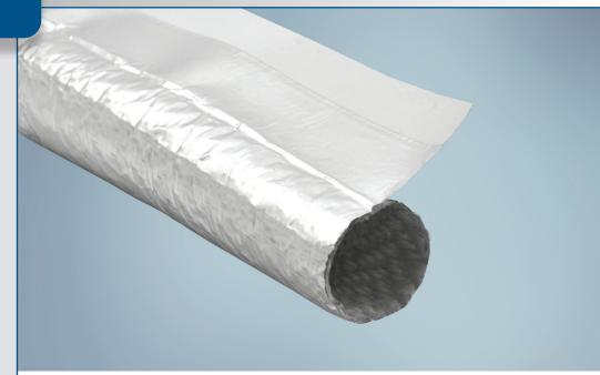
**ReflexWrap™ 1463** is a self-wrapping, reflective sleeve designed to provide thermal protection for both radiant and convective heat applications. Composed of a woven fiberglass base fabric and a lamination of aluminum foil, the product can withstand convective heat soaks up to +200°C (+392°F) and simultaneously protect critical components from radiant or reflected heat.
