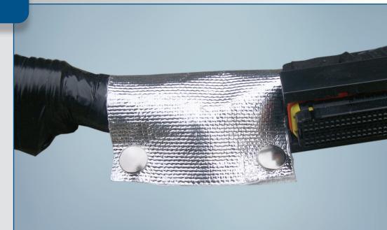
**ReflectSnap® 1420 HD** is a flexible, aluminized, wrappable sleeve designed to protect components in high temperature areas. The outer aluminum finish is highly reflective while the inner layer of fiberglass greatly increases insulating efficiency.
