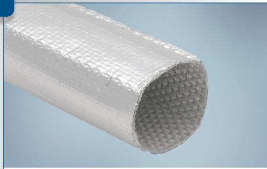
**ReflectSleeve® 1450E** is a woven, one-piece fiberglass sleeve that is bonded with an aluminized heat-seal film using a polymeric adhesive. A special manufacturing process permits the sleeve to boast a virtually seamless construction.
