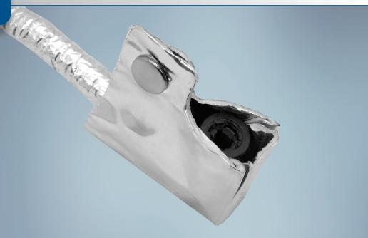
**ReflectShield® 1440P** is a three-layer composite system designed to provide excellent protection for components that must survive in high temperature areas. Aluminum is used as the outer layer for reflectance of radiant heat while the second inner layer utilizes polyester for insulation. The third layer can be a pressure sensitive adhesive (PSA) or a second layer of aluminum. The resulting product can then be slit to width and length or die cut into complex geometric shapes.
