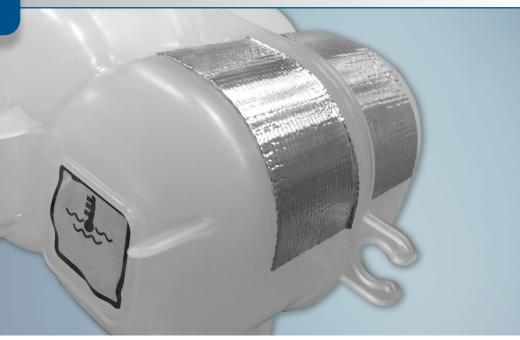
**ReflectShield® 1435SA2** is a woven fiberglass fabric with aluminum foil laminated to its outer surface and a pressure sensitive adhesive to its inner surface. This peel and stick laminate provides superior radiant heat protection for a variety of components including areas of complex geometry or difficult fixation.
