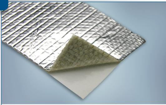
**ReflectShield® 1435** is a woven fiberglass fabric with aluminum foil laminated to its outer surface and a pressure sensitive adhesive to its inner surface. This peel and stick laminate provides superior radiant heat protection for a variety of components including areas of complex geometry or difficult fixation.
