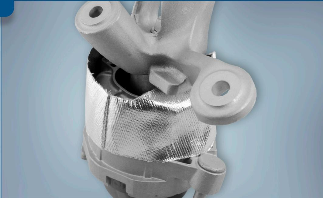
**ReflectShield® 1412** is a woven fiberglass fabric that has an aluminum foil laminated to its outer and inner surfaces. ReflectShield 1412 is designed to provide radiant heat protection for tubes, hoses, wire harnesses and other engine components.
