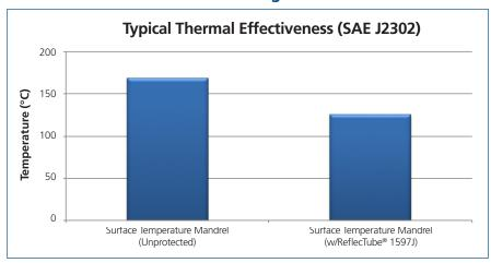
Note: Mandrel is parallel to and 25mm (1") away from a 550°C heat source
