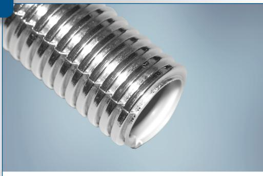
**ReflecTube® 1592** is a reflective convolute sleeve designed to provide thermal protection for components in radiant heat environments. Composed of a high temperature nylon 4,6 polymer base substrate and a highly reflective coating, ReflecTube 1592 provides protection for wires, cables and hoses in applications that have radiant heat source temperatures as high as +538°C (+1000°F).
