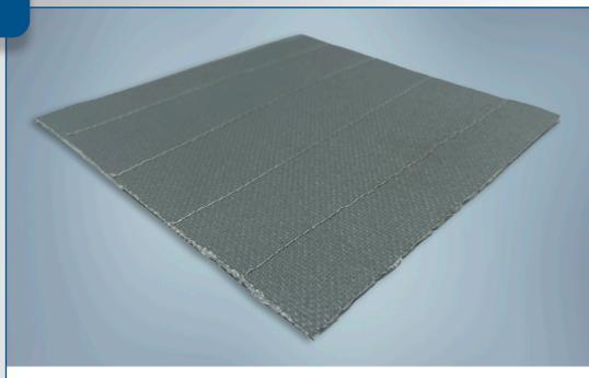
**Protexx-Shield® 7015** is a thin, flexible thermal and flame barrier specifically designed as anti-propagation protection within EV battery pack. Product is comprised of multiple layers of an engineered composite structure. Protexx-Shield 7015 acts as a flame barrier, low level blast barrier, medium level of thermal insulation and provides electrical insulation. Protexx-Shield 7015 is compatible with pressure sensitive adhesive to allow for direct application onto a variety of surfaces.
