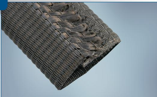
Hookit™ is a lightweight, damage-resistant sleeving used to protect and dress wiring and hose assemblies. Its patented hook and integral loop closing feature eliminates the need for an open end for installation. Hookit oversleeve permits quick and easy access for inspection, rework or replacement of components.
