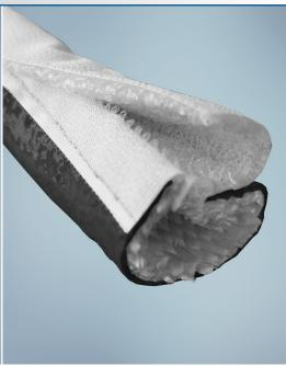
**FyreJacket® HL** is an open thickwall braided fiberglass sleeving coated with a specially compounded, flame retardant silicone rubber. FyreJacket HL can be easily installed on cables and hoses and closes thanks to the textile hook and loop structure.
