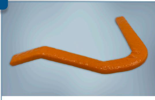
**FyreJacket® BP-A** sleeve is a highly expandable fiberglass structure with engineered silicone coating, providing superior flame protection and dielectric resistance. Product is specifically designed as anti-propagation protection in case of Thermal Runaway to ensure a good insulation & performance between the Battery Management Systems & the battery pack.
