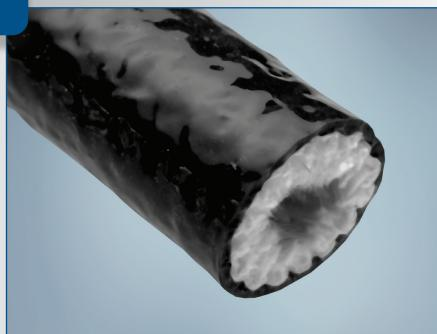
**FyreJacket® 1610** is a thickwall braided fiberglass sleeve coated with silicone rubber that provides thermal protection. FyreJacket 1610 is used to protect hoses, lines and cables in high temperature areas. It additionally provides protection against short-term hazards such as flame blasts. When burn-through is a threat, the specially designed sleeve construction retards the penetration of the flame. This can allow critical components to continue to function for a short amount of time.
