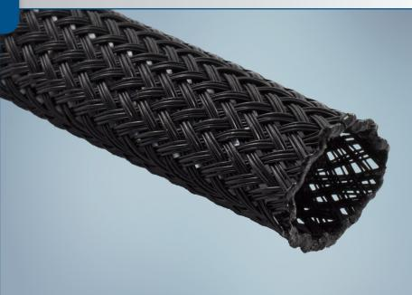
**FlexGuard® 2120** is a lightweight and flexible braided sleeve designed to provide mechanical protection for most common automotive applications. Constructed of PA (polyamide) monofilament guard strands and PET (polyethylene terephthalate) support strands, this dual-monofilament blend provides an excellent balance of abrasion protection, temperature resistance, and installability.
