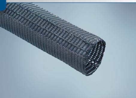
**FlexWrap® 2300** is a lightweight sleeve with a unique hook and loop self-closing feature that eliminates spot taping and does not require an open end for installation. The sleeve and integral loop portion of the closure system are manufactured entirely of polyester (PET) materials. FlexWrap 2300 permits easy access for inspection, rework or replacement of components.
