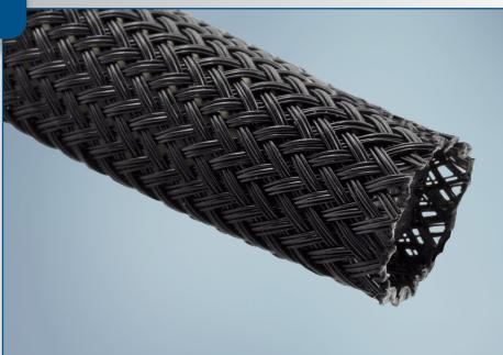
**FlexGuard® 2131** is a flexible, expandable sleeve that is both lightweight and rugged. Densely constructed of polyester, FlexGuard 2131 is specifically designed for the abrasion protection of automotive hoses, tubings and cables located in the engine compartment.
